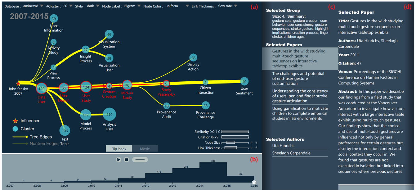
Fig. 2. Eiffel user interface: (a) Flow map for IGS; (b) Animation controller for evolutionary visualization; (c) The selected node group, which represents a list of nodes; (d) Detail panel on the selected node.
