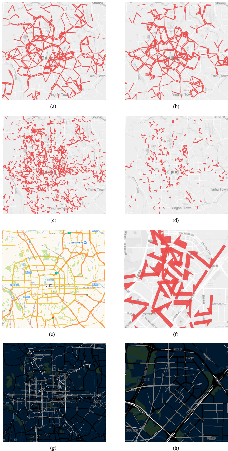
Fig. 2: Visual comparison of FlowMap and UrbanMotion on the same sparse trajectory data set: (a) abstract overview by FlowMap without map-matching ( MaxRadius = 3km ); (b) abstract overview by FlowMap using map-matched movement vectors as input data ( MaxRadius = 3km ); (c) more fine-grained visualization by FlowMap ( MaxRadius = 1km , without map-matching); (d) filter to show top 20% flows ( MaxRadius = 1km ); (e) the road network of the city of Beijing; (f) local movements in the Wangjing district by FlowMap using map-matching; (g) abstract overview by UrbanMotion without map-matching; (h) local movements by UrbanMotion using map-matching.
